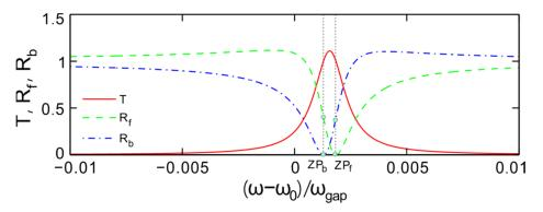
**Figure 2.** Transmittance and reflectance varying with the normalized frequency, respectively. Two lights are normally incident from the left and right, respectively. The gain–loss factor is q = 5.
