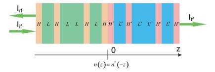
**Figure 1.** Schematic of PT-symmetric Cantor photonic crystal. The Cantor photonic crystal is composed of two  $S_2$  dielectric multilayers submitted to the Cantor sequence substitution rule and the two  $S_2$  of Cantor photonic crystal are symmetric about the center.
