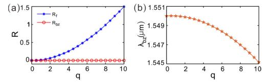
**Figure 5.** (a) Left reflectance varying with the gain–loss factor at the right-reflectionless incident wavelength. (b) Right unidirectionally invisible wavelength changing with the gain–loss factor.
