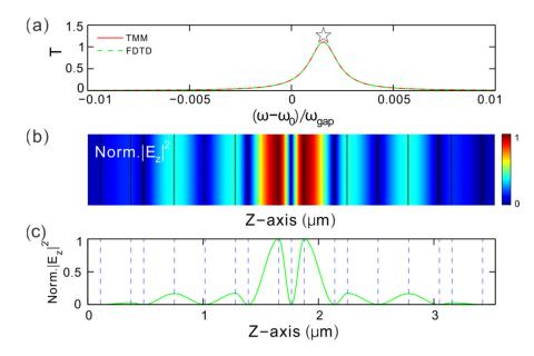
**Figure 6.** (a) Transmission spectra for the normally incident light waves for q = 5 in two different simulating methods. (b,c) Electric field distribution of the transmission mode simulated by TMM and FDTD, respectively.
