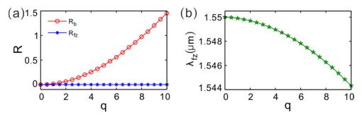
**Figure 4.** (a) The right reflectance varying with the gain–loss factor at the left-reflectionless incident wavelength. (b) The left unidirectionally invisible wavelength changing with the gain–loss factor.
