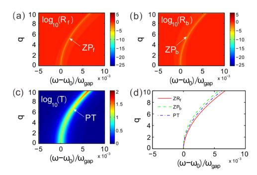
**Figure 3.** (**a**,**b**) Reflectance for lights incident from the left and right, respectively. (**c**) Transmittance of light in the parameter space. (**d**) Zero point of reflection and peak point varying with the normalized frequency and gain–loss factor.
