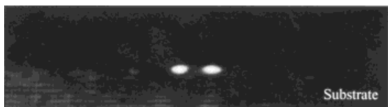
Figure 6 Near optical image coming out from the Y-branch waveguide for 1.55 \mu\text{m} light
