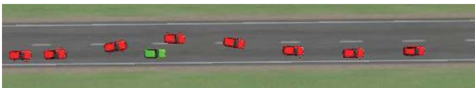
Figure 7. Collision avoidance maneuver of MPC control
