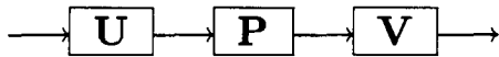
Fig. 1. Prototype unitarily equivalent system: P represents a traditional analysis/processing system, whereas U and V are unitary transformations [24].
