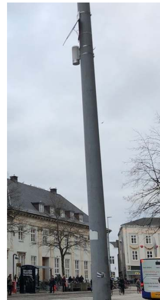
Figure 4. Station 16 in the sensor network mounted with a MONTEM CityProbe. The height of the CityProbe should be at least 4 meters.
