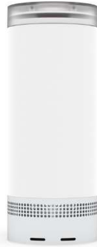
Figure 2. The MONTEM CityProbe. The height of the probe is 192 mm and the diameter 75 mm. It is made from hard plastic and light metals and weighs 558 g. The power supply comes from a solar panel attached by a cable.
