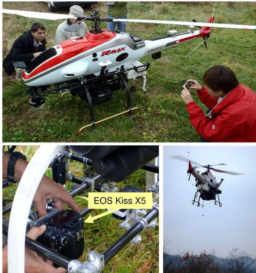
Figure 3. UAV (RMAX-G1) equipped with a digital camera (EOS KISS X5). doi:10.1371/journal.pone.0109881.g003
