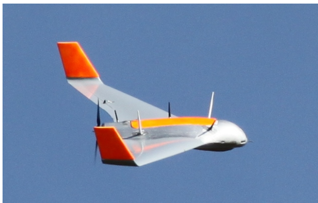
Fig. 3. Picture of X8 UAV with location of antennas used in the field test. The two white antennas are the 2.4 GHz WiFi antennas, while the others are two 5.8 GHz antennas for the AirMax wireless UAV-to-ground station data link, and one 433 MHz antenna for the UAV telemetry.
