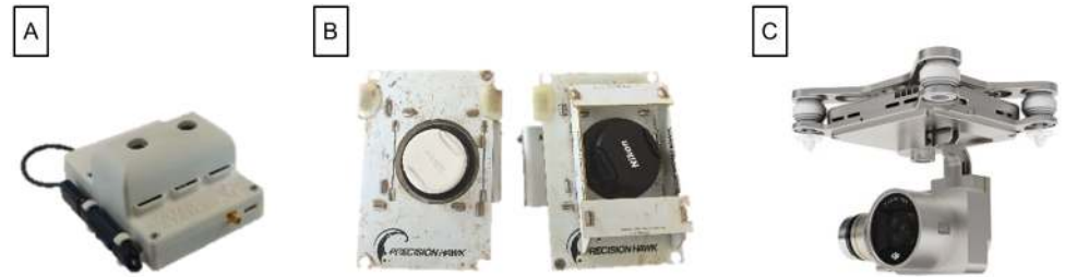
Fig 6. Sensors carried by the UAVs used in this study. (A) Sentek GEMS multispectral camera carried by the Anaconda fixed-wing UAV. (B) Nikon J3 digital camera (left) and modified multispectral camera (right) carried by the Lancaster fixed-wing UAV. (C) DJI P3-005 4K camera carried by the X88 octocopter.
