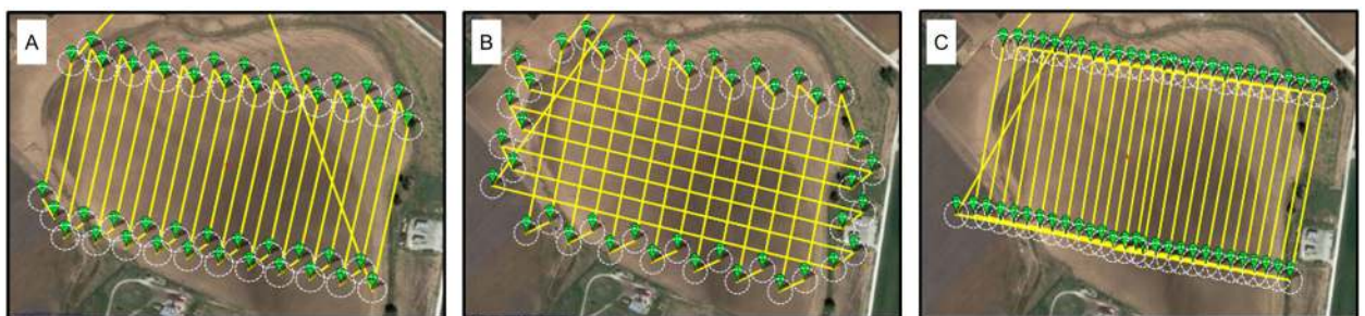
Fig 8. Three different flight paths over a 30-ha route pack evaluated by Anaconda fixed-wing UAV in this study. (A) Standard parallel flight path. (B) Cross-stitch flight path. (C) Moving-box flight path. The yellow lines represent planned flight paths; the green balloon-shape icons represent waypoints along the flight path for GPS navigation.
