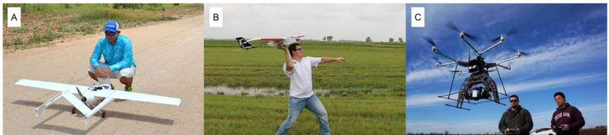
Fig 5. External physical characteristics of UAVs used in this study. (A) RMRC Anaconda fixed-wing vehicle. (B) PrecisionHawk Lancaster fixed-wing vehicle. (C) TurboAce X88 octocopter with autopilot computer interface (left), multiple battery options (middle), and navigation and gimbal transmitters (right). The individuals appearing in these figures gave written informed consent (as outlined in PLOS consent form) to publish these pictures.
