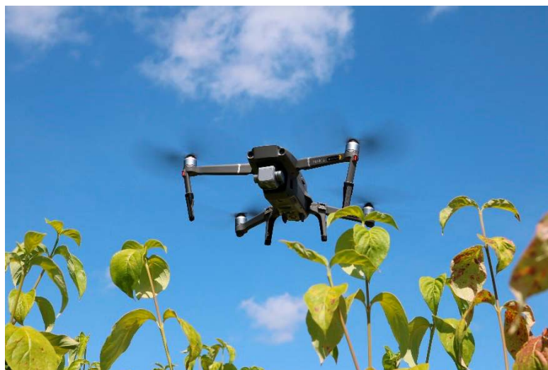
Figure 1. Example DJI Mavic 2 platform being used in a project at the Tennessee State University (TSU) Otis L. Floyd Nursery Research Center in McMinnville, TN involving automatic detection of biotic and abiotic stresses in nursery field productions. This unmanned aerial vehicle (UAV) platform will be equipped with a Raspberry Pi, 3D camera, and a multispectral camera to make up the unmanned aircraft system (UAS).
