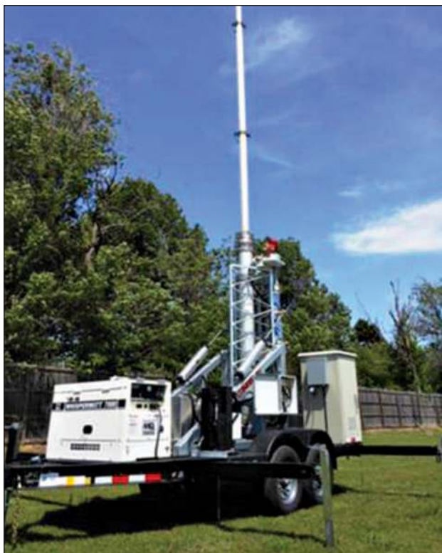
FIGURE 2 The transportable tower and GS.
