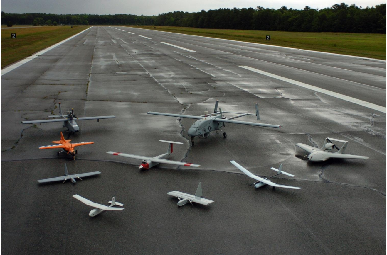
Figure 7. LASE and LALE UAS on display at 2005 Naval Unmanned Aerial Vehicle Air Demo. Pictured are (front to back, left to right) RQ-11A Raven, Evolution, Dragon Eye, NASA FLIC, Arcturus T-15, Skylark, Tern, RQ-2B Pioneer, and Neptune. Image Courtesy US Department of Defense.
