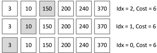
FIGURE 2—A client wishing to retrieve an item with label “3” from a server holding a sorted list of 6 items would need to perform three rounds of probing. During each probe, the client guesses an index, uses PIR to retrieve the (label, c) -tuple at that index, and refines the guess accordingly. “Cost” indicates the number of items processed by the server in each probe.
