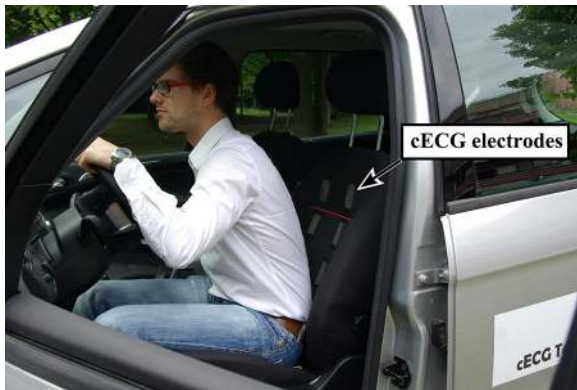
Figure 2 Picture of a driver sitting in the car seat with the integrated electrodes.
