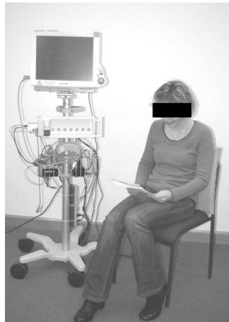
Figure 1 Picture of a patient sitting on the chair equipped with the cushion and the integrated cECG electrodes.
