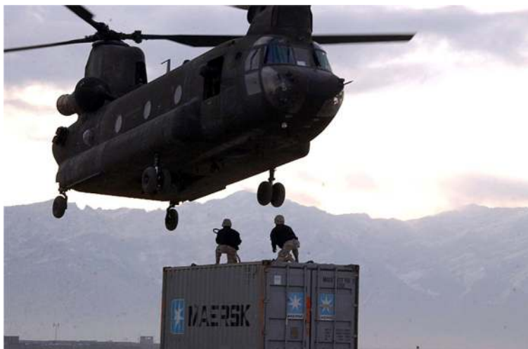
Figure 3 Chinook transport helicopter—payload 12,000 kg; range 1,100 km.
