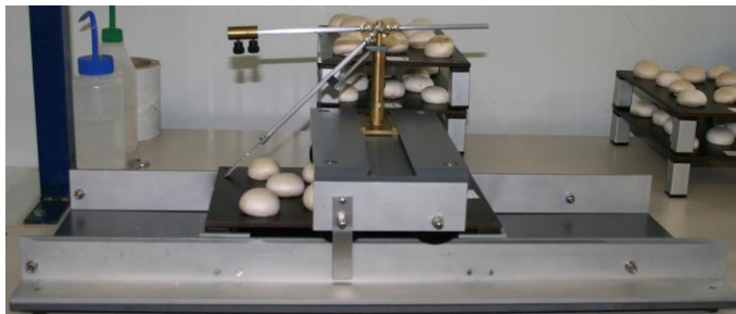
Figure 1. Bruising device. The black tray can hold ten mushrooms, with the stem placed through the hole. The spatula can be moved by hand over the tray. The weights on the horizontal bar can be adjusted.
