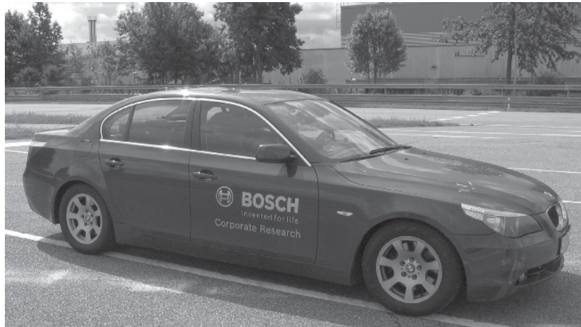
Figure 11. Conventional BMW 5 Series serves as the test vehicle for the proposed UKF state estimation concept.
