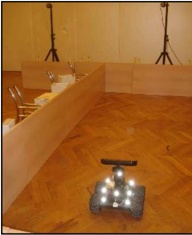
Fig. 1: Testing arena with Wifibot robot in the foreground of the picture. We can also see two of the seven Optitrack cameras in the background.
