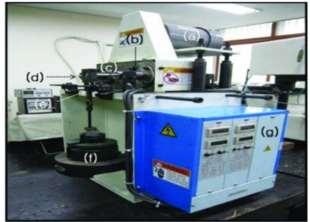
Fig. 11 Cantilever type fatigue testing machine, (a) motor, (b) specimen, (c) stopper, (d) bearing, (e) hanger, (f) weight, (g) counter
