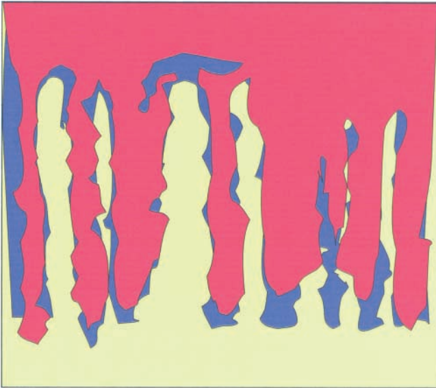
Fig. 4. Superposition of the draining front 16 min into the third cycle (blue), and 18 minutes into the fourth cycle conducted 28 d later in the same column. (red)
