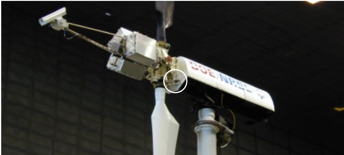
Figure A-17. Rotor lock installed for parked blade sequences L and O
