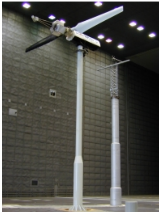
Figure G-2. Full view of UAE turbine and wake measurement tower in (80 x 120) test section
