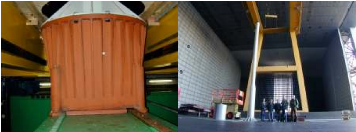
Figure 3. NASA semi-span mount and wind turbine tower in 24.4-m x 36.6-m test section
