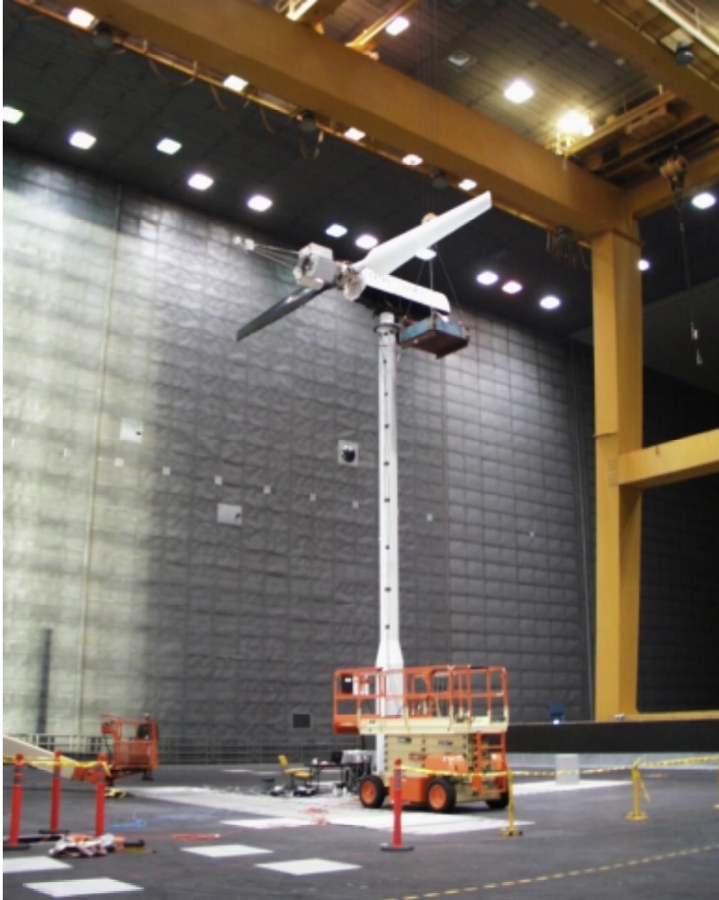
Figure A-18. Steel reaction mass suspended from gantry crane
