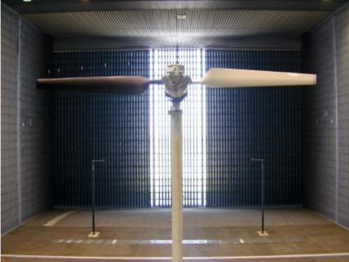
Figure 4. Inflow velocity and flow quality measurements upwind of the turbine. Total pressure and static pressure ports are located on walls, ceiling, and floor (obstructed by tower) of wind tunnel. Sonic anemometers were mounted on airfoil-shaped stands.
