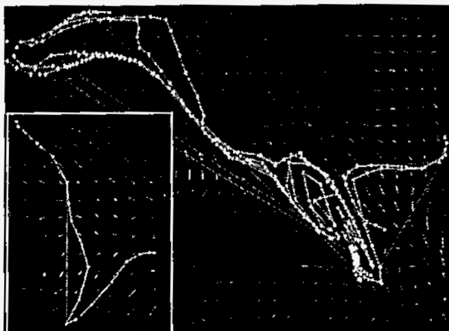
Figure 4. The orange streakline has particles adaptively added and deleted as determined by segment length. The purple streakline does not. The inset shows an earlier frame in the animation.
