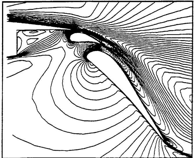
Figure 13 Computed Mach Contours for Flow Over Four-Element Airfoil Configuration Mach = 0.1995, Reynolds Number = 1.187 million, Incidence = 16.02 degrees
