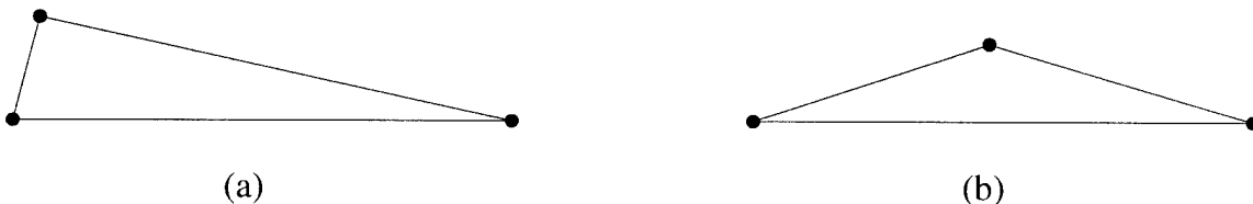
Figure 27: Illustration of two types of high aspect ratio triangles: non-obtuse (a) and obtuse (b).
