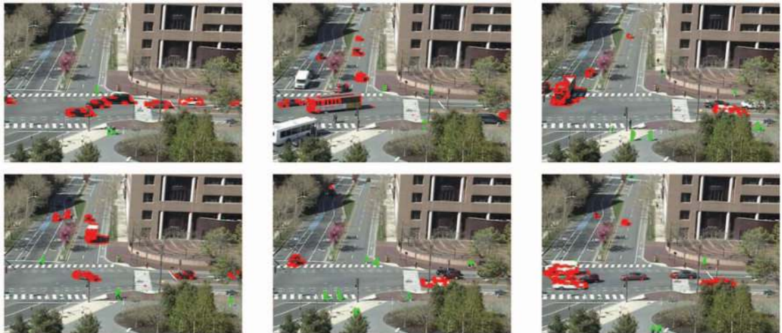
Fig. 14. Vehicle and pedestrian detection. Vehicle motions are marked by red color and pedestrian motions are marked by green color.
