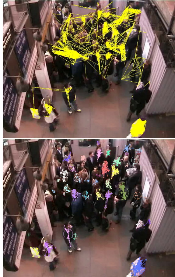
Figure 9. Sequence subway-B152 is a minute long and features our most dense pedestrian traffic. (A) Pairs of features with high likelihoods of being joined. (B) Isolated groups of features result from applying the discriminant function. Please view the video results for an excerpt of the sequence.
