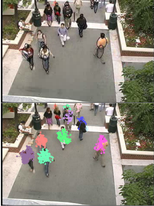
Figure 7. Frame 540. Example results from Zhao and Nevatia’s multiple-human tracker [32] (above) on their Commons01 sequence, and the results of our independent-motion detection. Note different false negatives in both. See video for entire sequence.
