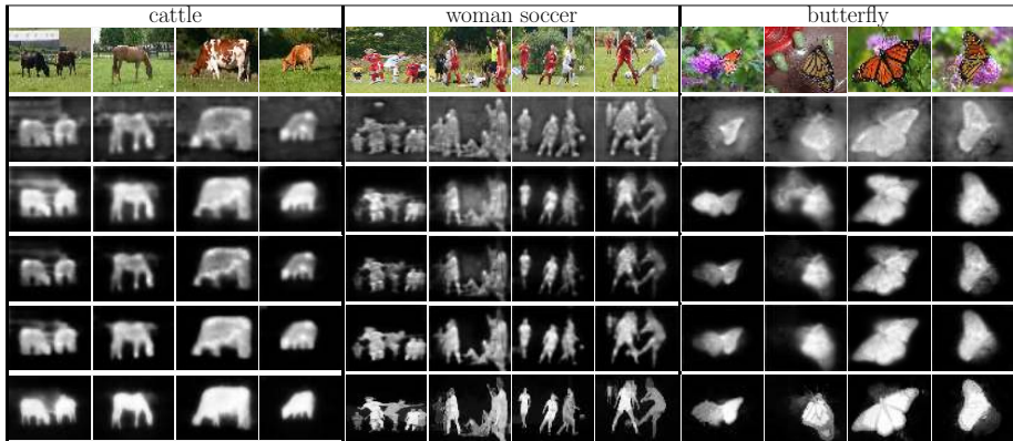
Fig. 6. Example co-saliency maps generated by combinations of different components. From the top to the bottom, they are the given images, g_c , g_s , g_c+g_s , g_c+g_s+g_e and g_c+g_s+g_e+D , respectively.
