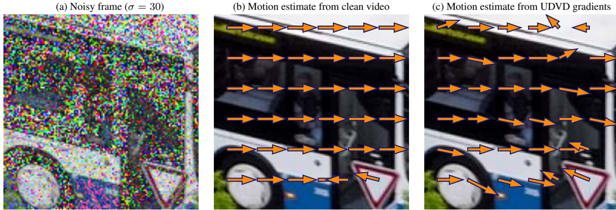
Figure 5. CNNs trained for denoising automatically learn to perform motion estimation. (a) Noisy frame from a video in the DAVIS dataset. (b) Optical flow direction at multiple locations of the image obtained using a state-of-the-art algorithm applied to the clean video . (c) Optical flow direction estimated from the shift of the adaptive filter obtained by differentiating the network, which is trained exclusively with noisy videos and no optical flow information. Optical flow estimates are well-matched to those in (b), but deviate according to the aperture problem at oriented features (see black vertical edge of bus door), and in homogeneous regions (see bus roof, top right).
