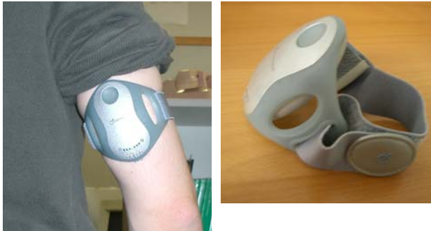
Figure 1. Wearing position and form factor of the SenseWear armband.
