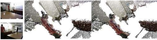
Fig. 3. Left: When a naive nearest-neighbor metric is applied, two sides of an object will be drawn toward each other, often at the expense of violating free space. Right: Our occlusion-aware energy term is able to recover from many of these situations.
