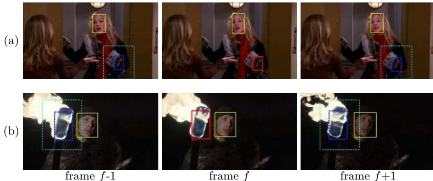
Fig. 2: Mining hard negatives from detector-flicker. The solid boxes denote detections, and the dashed boxes are associated with the tracking algorithm. Given all of the high-confidence face detections in a video ( yellow boxes), the proposed algorithm generates a tracklet ( blue dashed boxes) for the current detection ( red box in frame f ) by applying template matching within the search regions of the adjacent frames ( cyan dashed boxes). As there are no matching detections in adjacent frames for the current detection ( i.e. no yellow box matches the blue dashed boxes in frames f-1 or f+1 ), it is correctly considered to be an “isolated detection” and added to the set of hard negatives . The remaining detections in frame f , which are temporally consistent, are added to the set of pseudo-positives .
