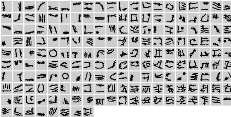
FIG. 18. Learned dictionary of templates from the Caltech-101 dataset in one run of an experiment, with 30 training images from each category. Template size is 64 \times 64 . Number of basis functions in each template is 15.
