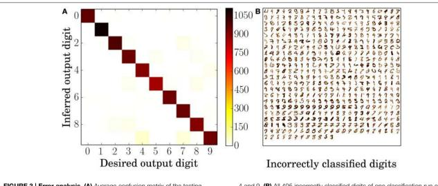
**FIGURE 3 | Error analysis. (A)** Average confusion matrix of the testing results over ten presentations of the 10,000 MNIST test set digits. High values along the identity indicate correct identification whereas high values anywhere else indicate confusion between two digits, for example the digits
