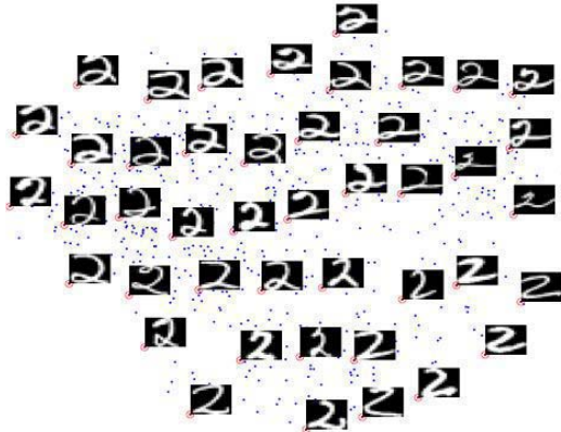
Figure 6. Results of SDE using k = 4 nearest neighbors on N = 638 images of handwritten TWOS. Representative images are shown next to circled points.
