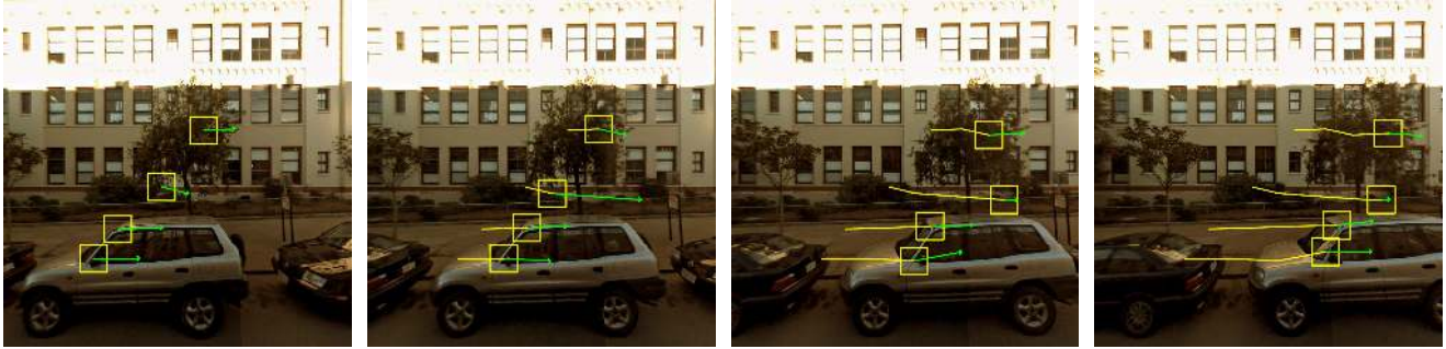
Figure 1. An example of corner feature tracking with optical flow. The video sequence moves frame-to-frame from left to right. The center of each yellow box in the left-most (first) frame is a corner detected by [22, 4]. The green arrows show the motion of these corners into the next frame as determined with optical flow [16, 4]. This is not a prediction. The flow algorithm uses the next frame in the sequence for this calculation. The yellow boxes contain the patches extracted and saved for later optimization. The yellow path tails in the subsequent frames depict patch movement as estimated by the optical flow. In total, four patch sets are produced, each with four patches. They are shown in Figure 2. Our algorithm produces additional patches for these frames. We do not show them for a simpler illustration.
