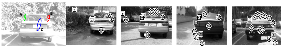
Fig. 5. Multiple use of parts: The three-part model on the left correctly classified the four images on the right. Part labels are: \circ = ‘A’, \square = ‘B’, \diamond = ‘C’. Note that the middle part (C) exhibits a high variance along the vertical direction. It matches several locations in the images, such as the bumper, license plate and roof. In our probabilistic framework, no decision is made as to the correct match . Rather, evidence is accumulated across all possible matches.
