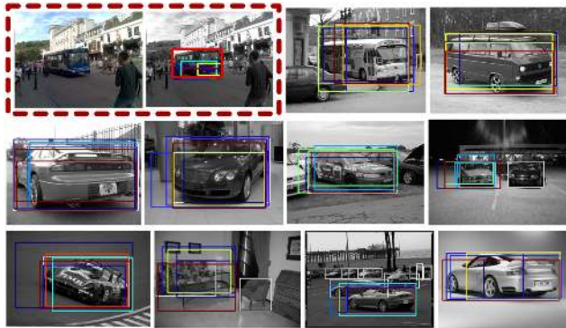
Figure 9. Localization in an example and its neighbor images on mixed-class PASCAL07-all. A bus is successfully localized in the image (red dashed box) from its neighbors (10 images) containing even other classes (car, sofa). Boxes in the neighbors show potential objects at the final iteration. (Best viewed in color.)
