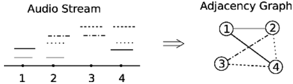
Fig. 6. Production of an adjacency graph from alignment paths and extracted nodes. The audio stream is shown as a timeline, while the alignment paths are shown as pairs of colored lines at the same height above the timeline. Node relations are captured by the graph on the right, with edge weights given by the path similarities.
