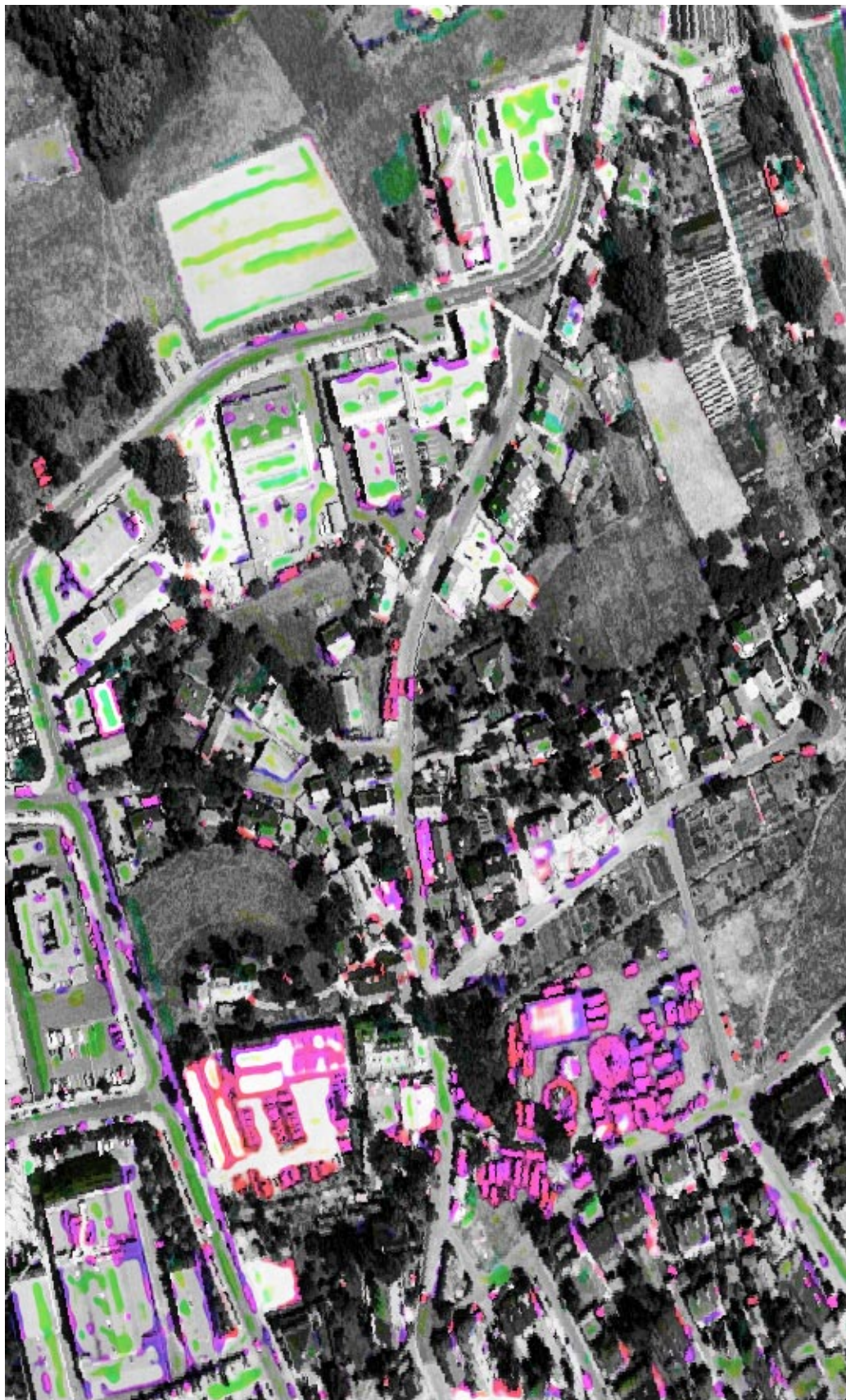
'Change' -image as detected from the temporal difference of logarithmic local variance, considering a small local neighborhood of 5 \times 5 pixels. The 'change'-hue codes the spectral 'direction' of change in the N -dimensional change space, while the magnitude of 'change' is coded in the color saturation ( i.e. , 'NoChange' has vanishing saturation and thus appears white or gray); the intensity values stem from one band of the underlying images.
