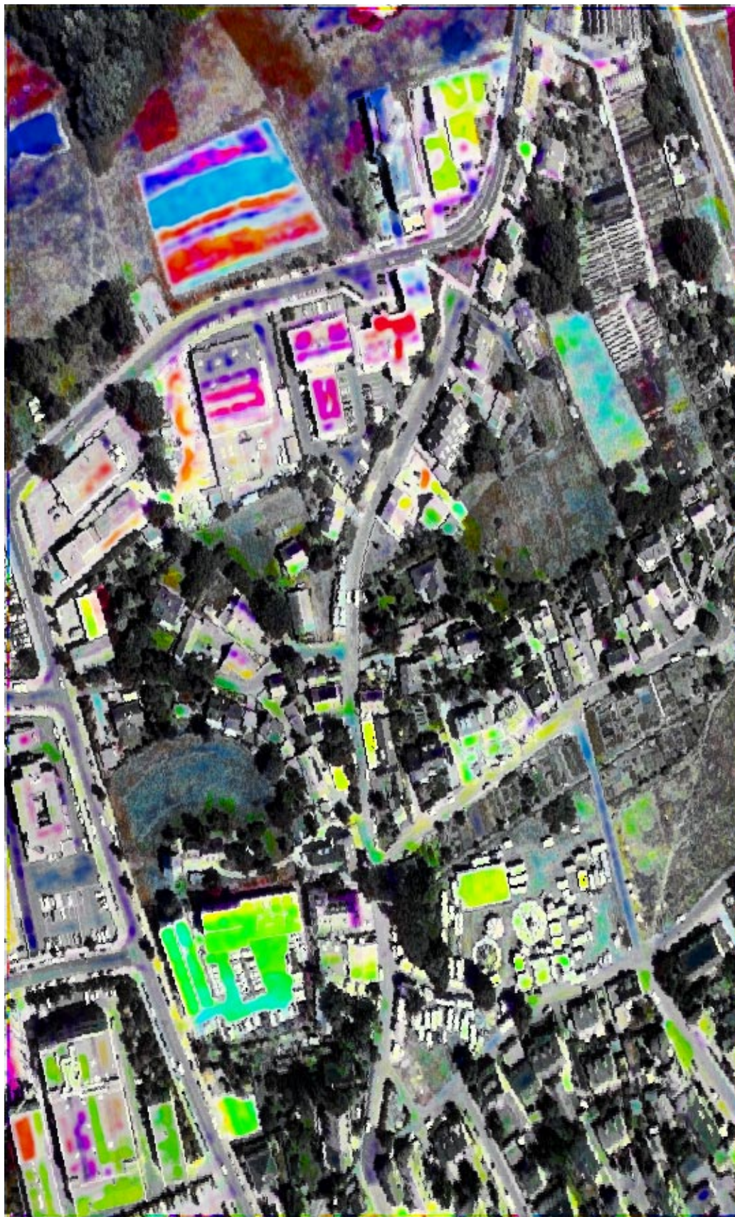
'Change' -image as detected from iterative principle component analysis (with local variance normalization c_i/\sigma_i ), considering a small local neighborhood of 5 \times 5 pixels. The 'change' -hue codes the spectral 'direction' of change in the N -dimensional change space, while the magnitude of 'change' is coded in the color saturation ( i.e. , 'NoChange' has vanishing saturation and thus appears white or gray); the intensity values stem from one band of the underlying images.
