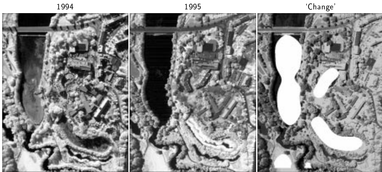
Figure 2: 'Change'-image (right, 800 \times 650 pixels) as detected from iterative principal component analysis, considering a large local neighborhood of 45 \times 45 pixels. 'Change'-areas are whitened.
