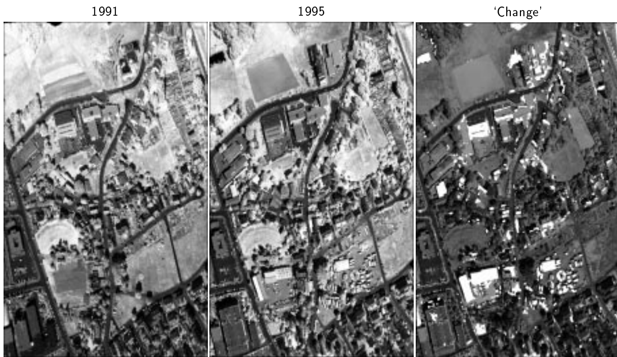
Figure 3: 'Change'-image (right, 900 \times 550 pixels) as detected considering a small local neighborhood of 5 \times 5 pixels. 'Change'-areas are whitened.
