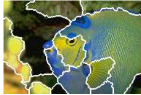
Fig 9. Example segmentation results on images from Corel photo CDs. 2,500 images are automatically processed without any parameter tuning on individual images (one scale, size 192 x 128 pixels).
