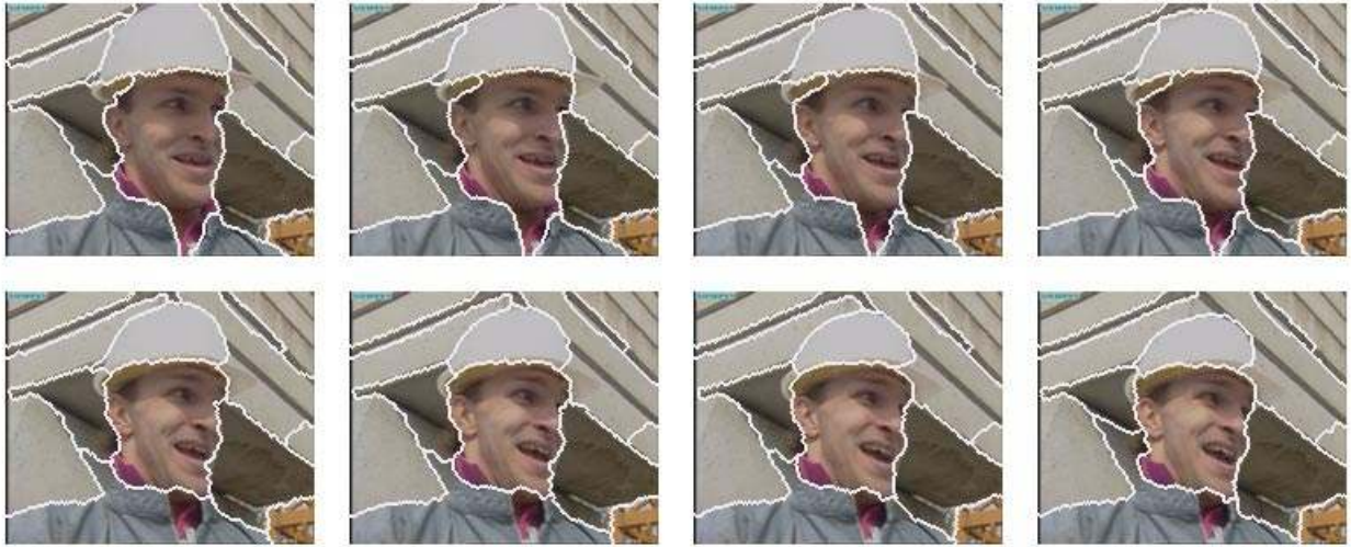
Fig 14. Segmentation results on the “foreman” sequence. Sample frames are chosen where large object motion occurs. (a) Frame 76-83. (b) Frame 127-134. The first 150 frames are segmented as a group and the minimum object duration is 15 frames or 0.5 s. Frame size 176 x 144.
