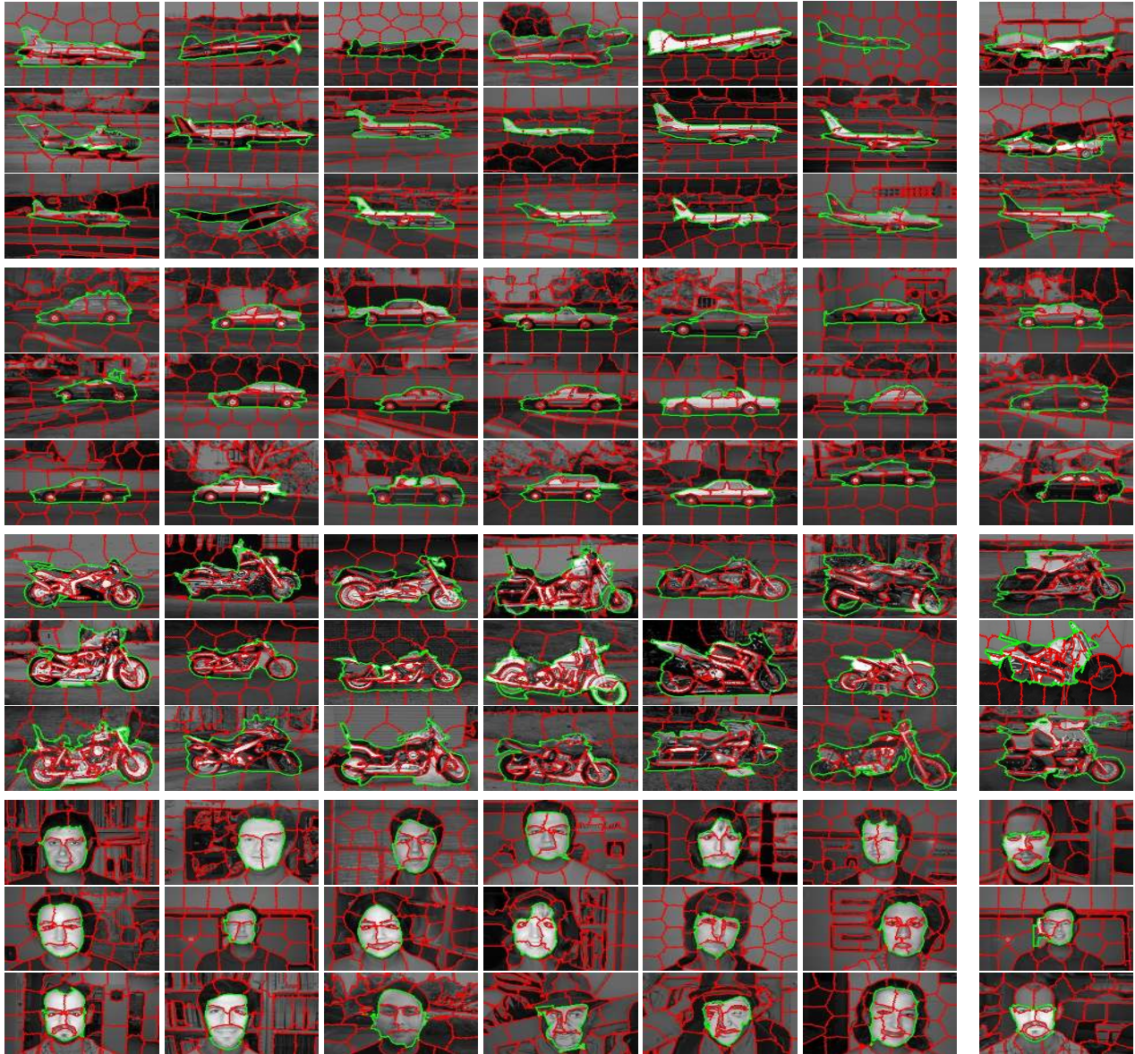
Figure 4. Segmentation results of our algorithm on example test images in standard datasets. Gray-scale images are used. The superpixel representation is shown in red and the final segmentation is shown in green . The brightness of the estimated background superpixels is diminished to aid visibility. We test the algorithm on Caltech faces, airplanes, motorbikes, and Caltech 101 cars. Note that the quality of segmentation is affected due to bad approximation of object boundaries by the superpixel boundaries. For most images the segmentation is quite accurate , even in the presence of intra-class variation and poor object-background contrast. Exemplar failures are shown in the last column . Performance for faces is low in table 1 because the unsupervised algorithm learned to segment faces without hair. This figure is most easily interpreted when viewed in color.
