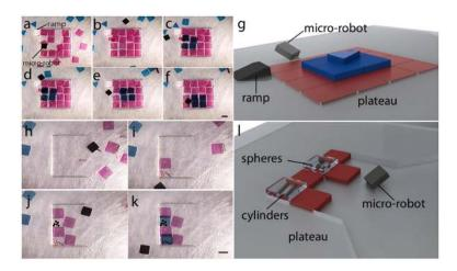
Figure 4. Three-dimensional micro-robotic coding of material composition
