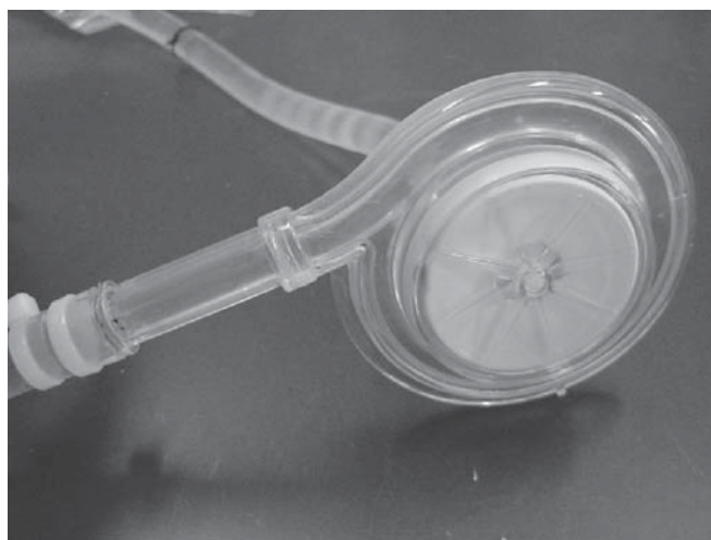
Fig. 3. The centrifugal pump after 151 days of perfusion. No thrombus formation was observed in the centrifugal pump except for minor amounts of thrombus formation on the edge of the shroud
