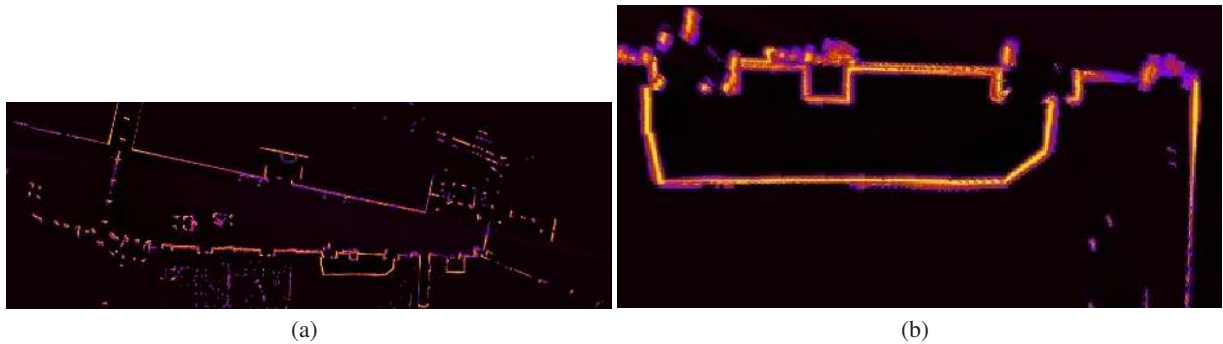
Fig. 1.4. Map from the Freiburg data set generated with the exponential forgetting policy and a initialization to an empty map. (a) Entire map (b) Zoom on the map.
