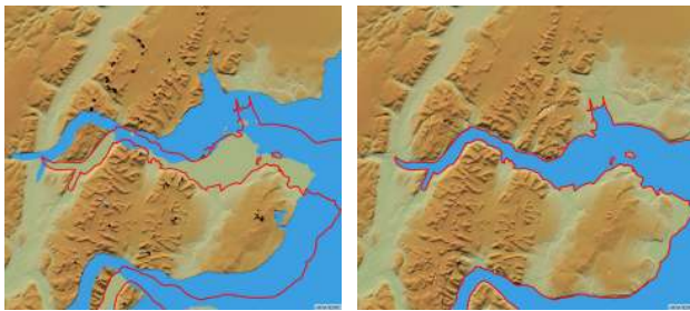
Figure 6. AW3D30 N80W016-021. Left: original, Right: sea masks corrected. Red lines and blue areas depict OSM coastlines and sea masks respectively.
