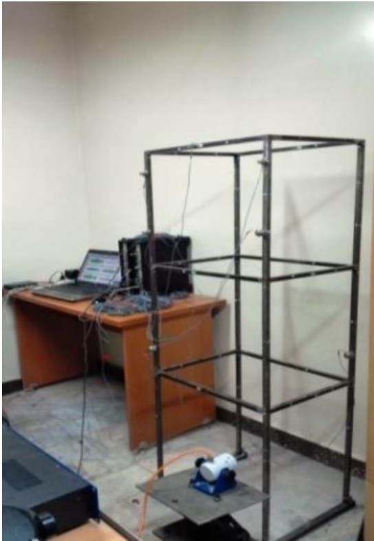
Figure 10: Equipment used in experimental modal analysis
