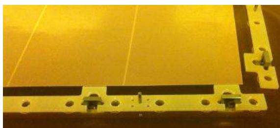
Figure 5. Close-up of the plastic frame for the manual stretching.
