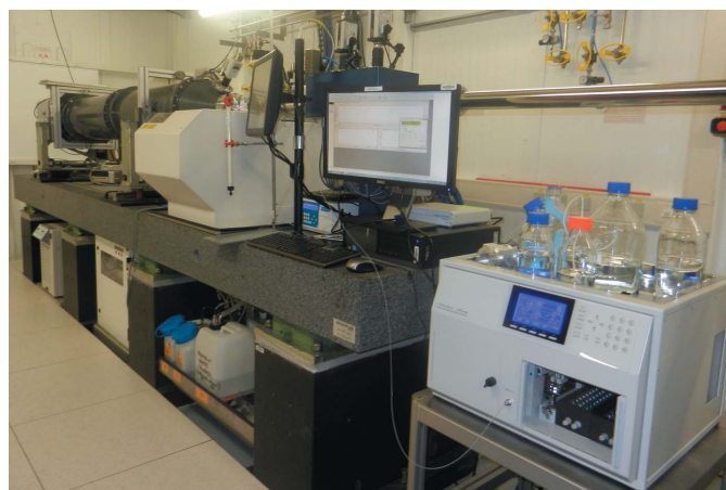
Figure 3 Experimental hutch set-up with HPLC and sample-changer units, slit box (blue), flight tube and detector at the back.
