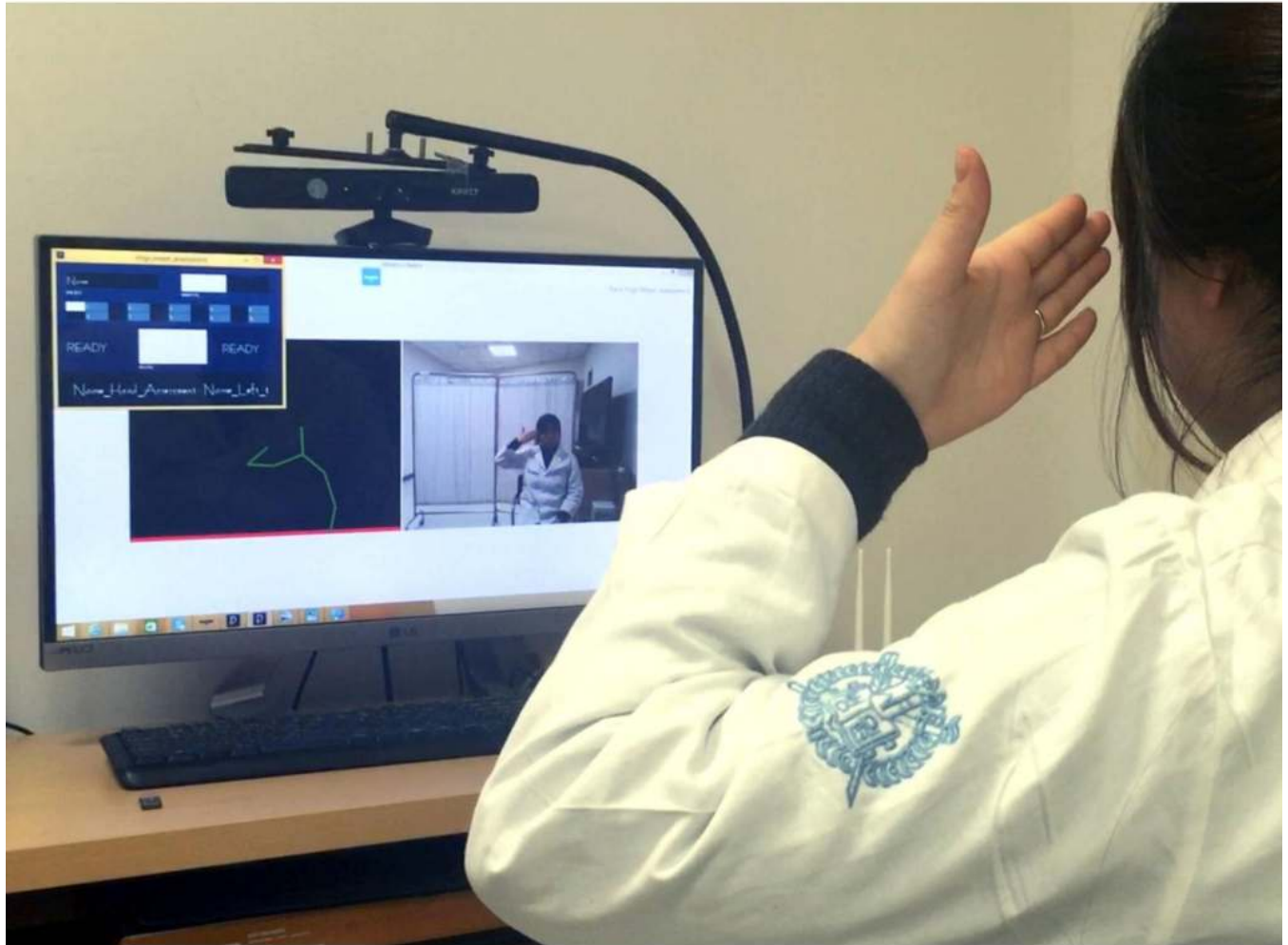
Fig 1. Motion data recording program. The recording program includes subjects' abbreviation, recording arm side, assessment item number. When pushing the record button and starting an item of Fugl-Meyer assessment, upper extremity skeleton of a subject can be shown in the monitor.
