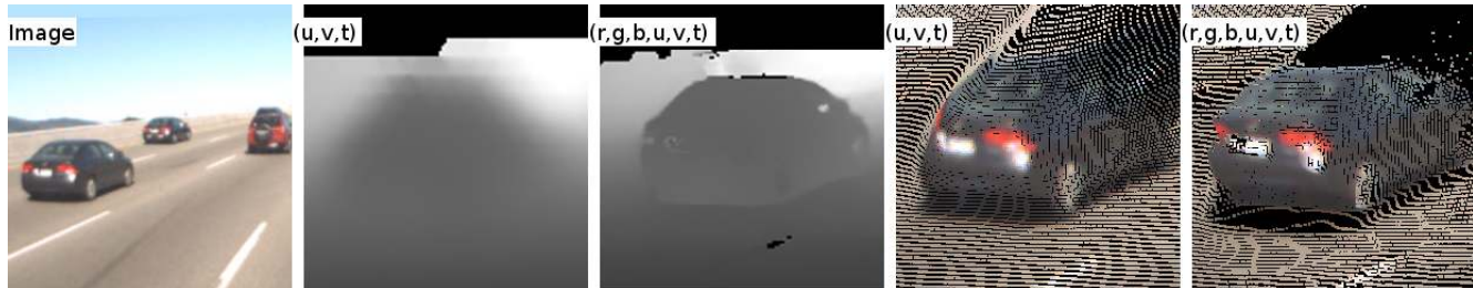
Figure 7. This figure compares depth maps generated by our algorithm with color information and without. We zoom in on the area of the depth map near the closest car; the first two columns show the depth map in that area, and the second two are 3D visualizations where each image pixel is offset by its corresponding value in the depth map. Without color information, blending occurs across depth discontinuities.
