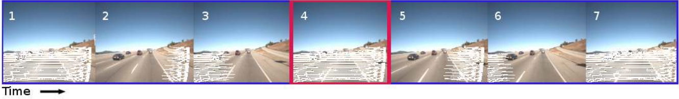
Figure 5. Here we show the input buffer used in our non-synthetic evaluations. The white points indicate pixels where both depth and color information is available. We hold out depth information from frame 4, bordered in red, and use only the surrounding depth information to generate a depth map at that frame. The depth information actually recorded at the time frame 4 was captured is then used to evaluate the quality of our generated depth map.
