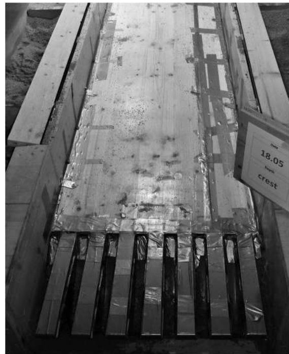
Fig. 6. PKW Configuration A (Table 1) and upstream channel with a fixed horizontal bed at elevation e/P = 0 equal to z = 0 m (Fig. 4).
